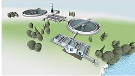
Fourth treatment stage: Typical process with HUBER Disc Filter RotaFilt® as downstream polishing filter: (1) PAC dosing, (2) Contact basin, (3) Sedimentation tank, (4) Polishing filter with HUBER Disc Filter RotaFilt®
