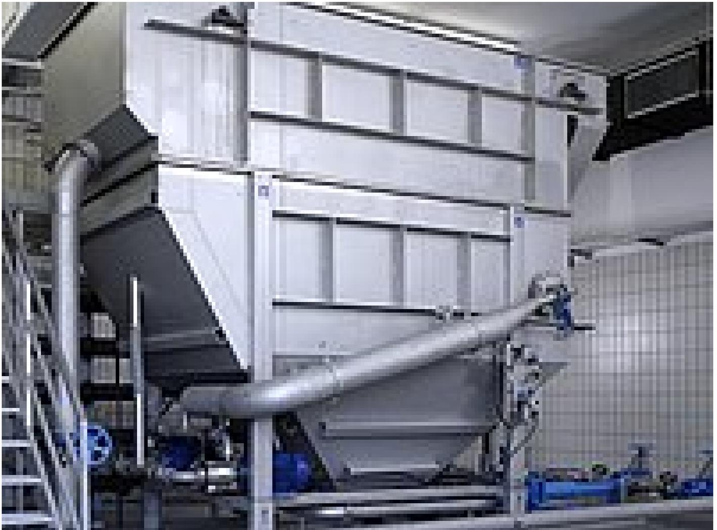
Effective and efficient wastewater and process water treatment for industrial applications through flotation with micro bubbles
