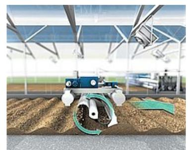
A double shovel is ploughing through the sludge bed and turning the sludge as the machine is moving through the greenhouse
