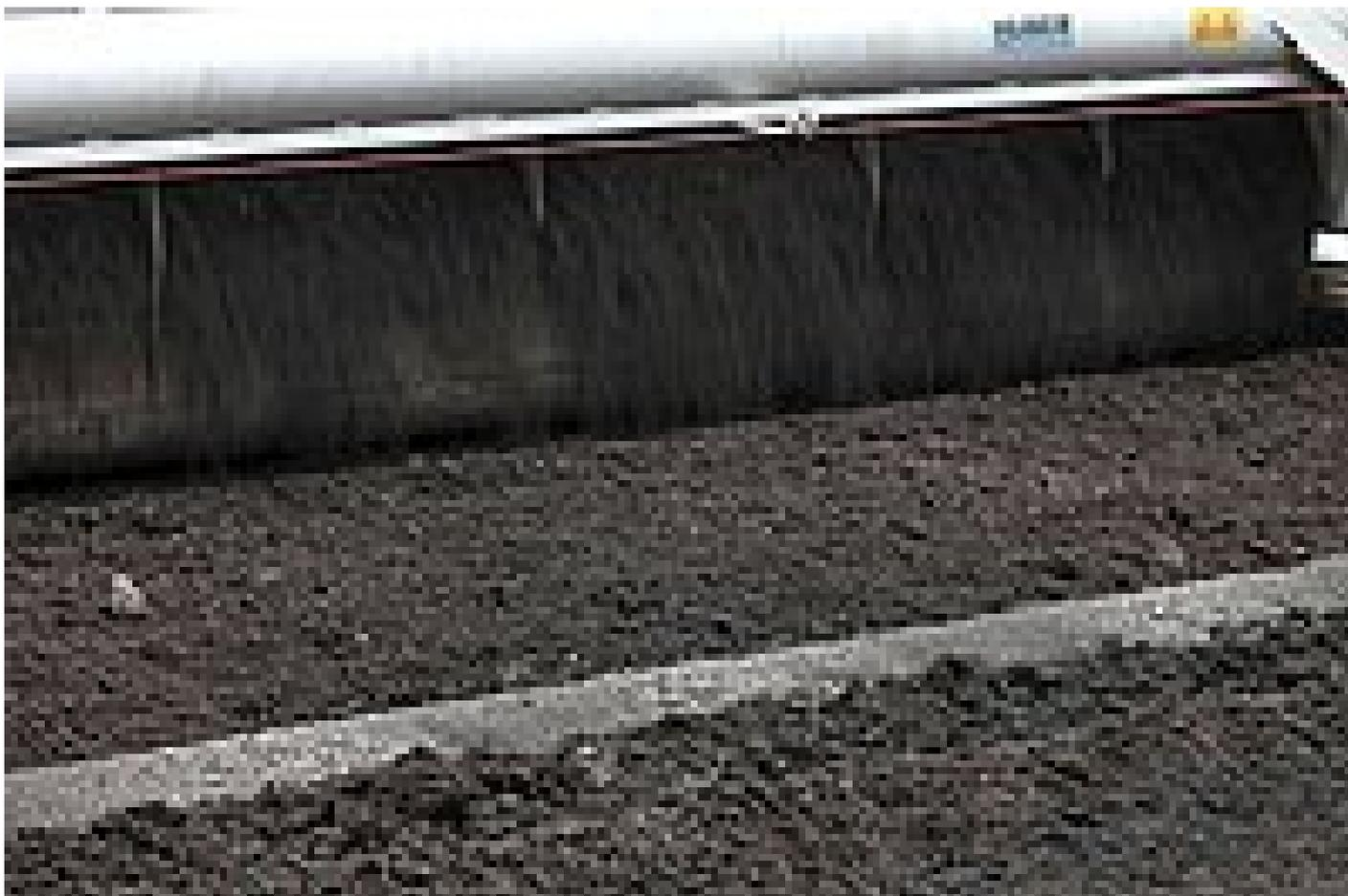
*Through backmixing of dry sludge granulate and sludge aeration the HUBER Solar Active Dryer SRT 9 provides the sludge bed conditions required for maximum drying results*
