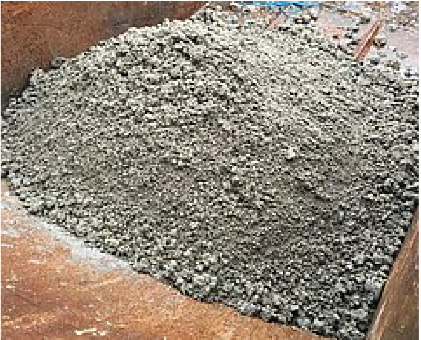
Dewatered sludge cake from the Q-PRESS®
