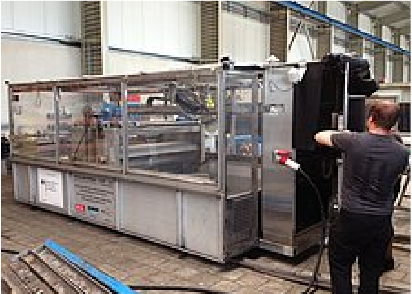
Comeback of the baby solar dryer: inspection of the electrical control system in the HUBER service factory
