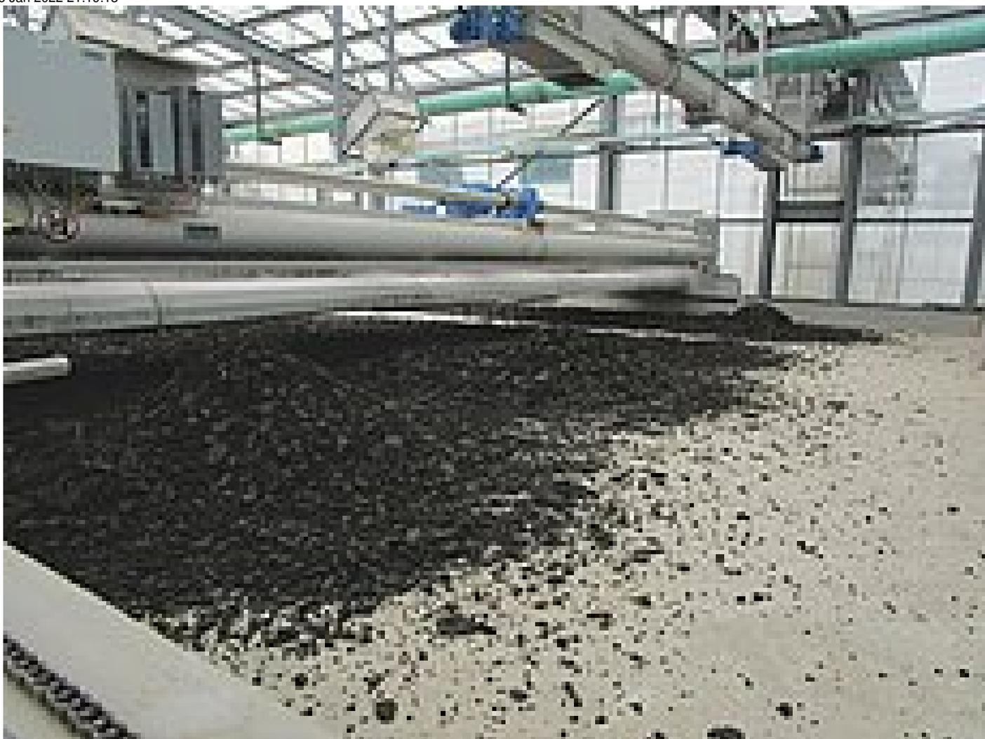
*The new SOLSTICE® 11 turning sludge at Zhenjiang, China*
