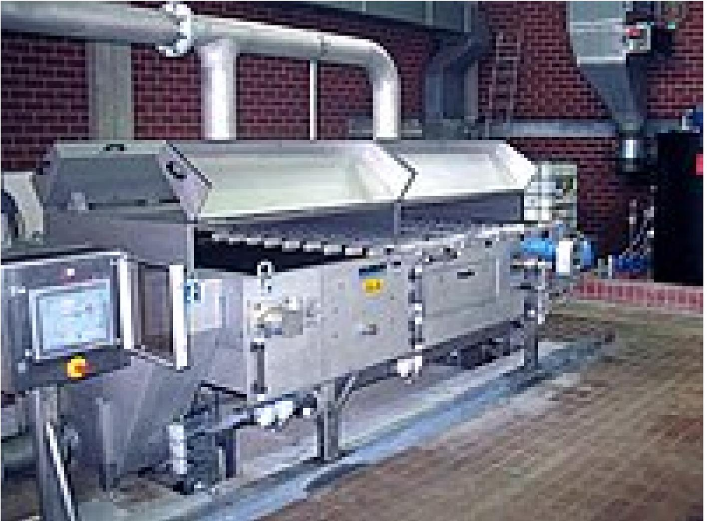
Large scale trials in direct comparison with competitors resulted in the order for the HUBER Belt Thickener Drainbelt DB being awarded to HUBER. The start-up results of the finally supplied and installed unit even exceed the guaranteed performance data and test results of the trial unit significantly. Since April the Drainbelt has proven its efficiency and minimized the operating costs for excess sludge thickening.
