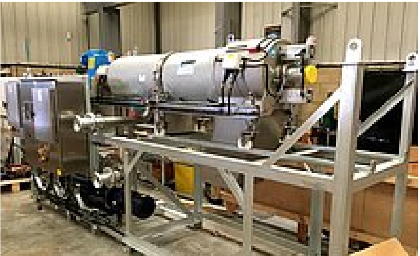
Figure 5 - Skid-mounted trial unit with feed pump & control panel
