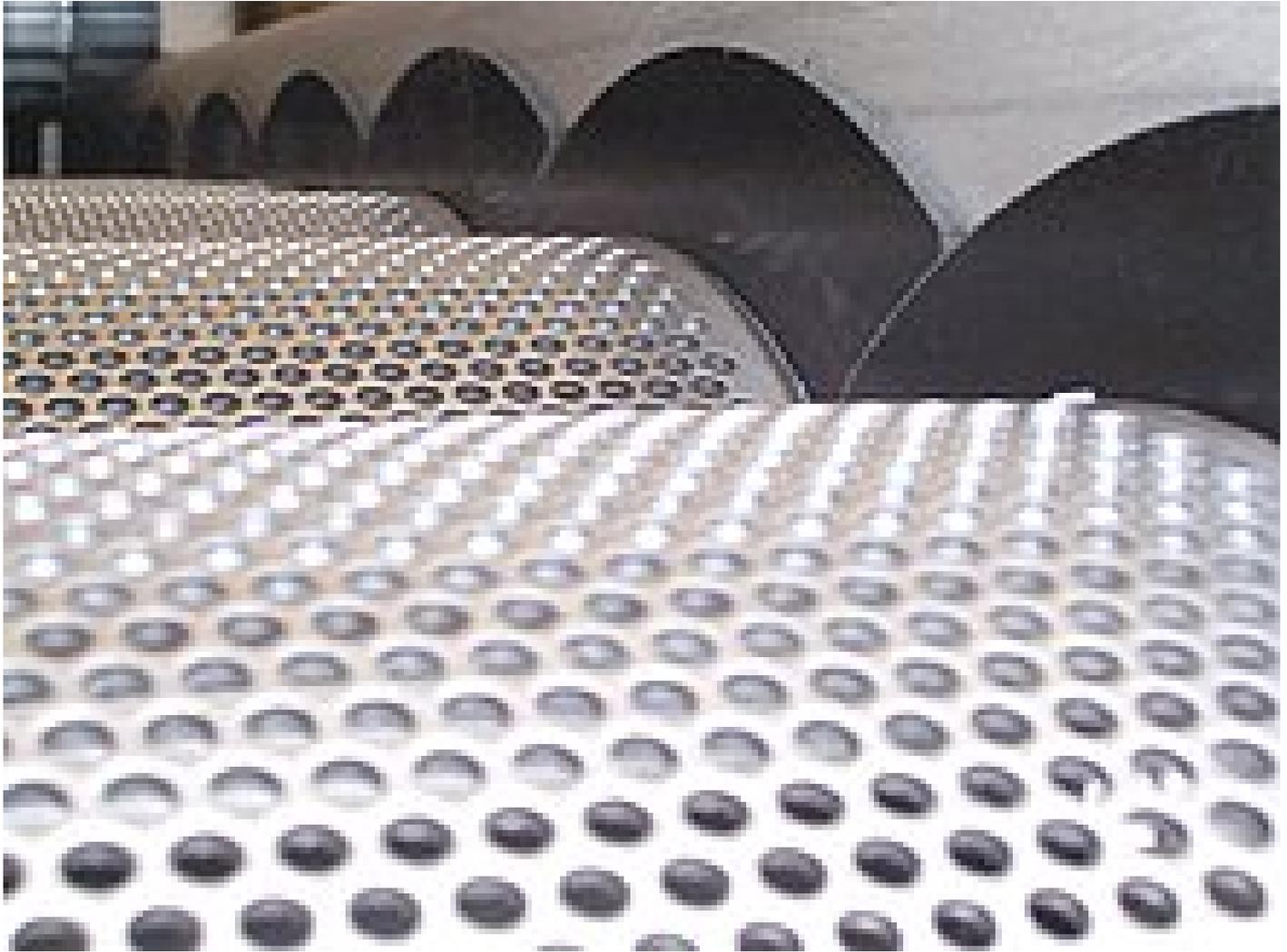
*Excellent separation efficiency due travelling perforated plates*
