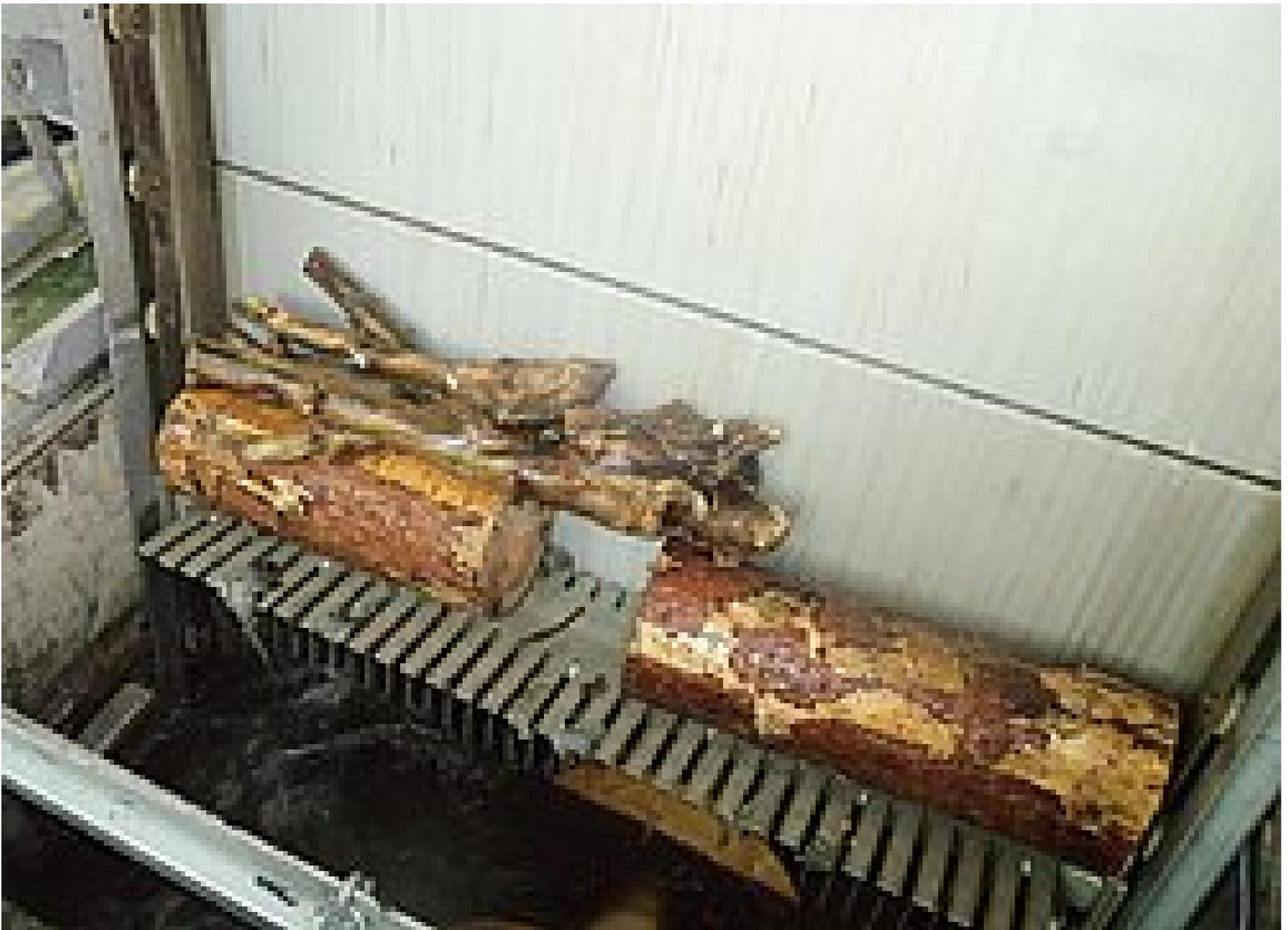
*Reliable removal of even bulky coarse material by the TrashMax® screen*
