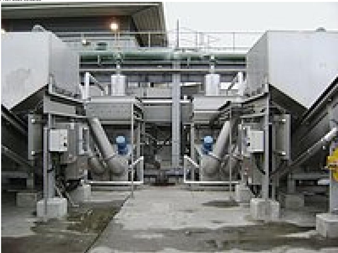
*Laundry tanks and rising compaction pipes of the seven WAP/SL units*
