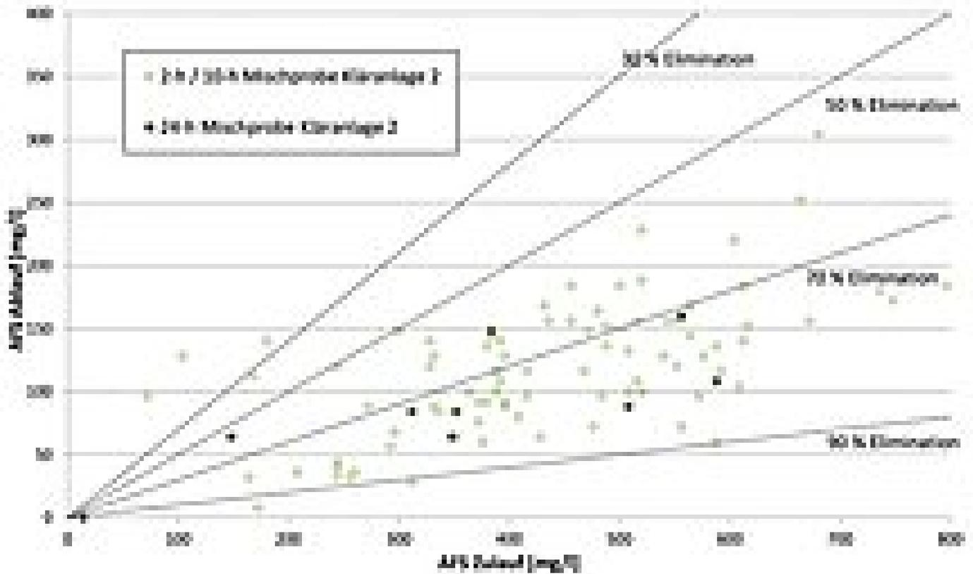
Reduction achieved for filterable solids with a plant size of 17,000 PE
