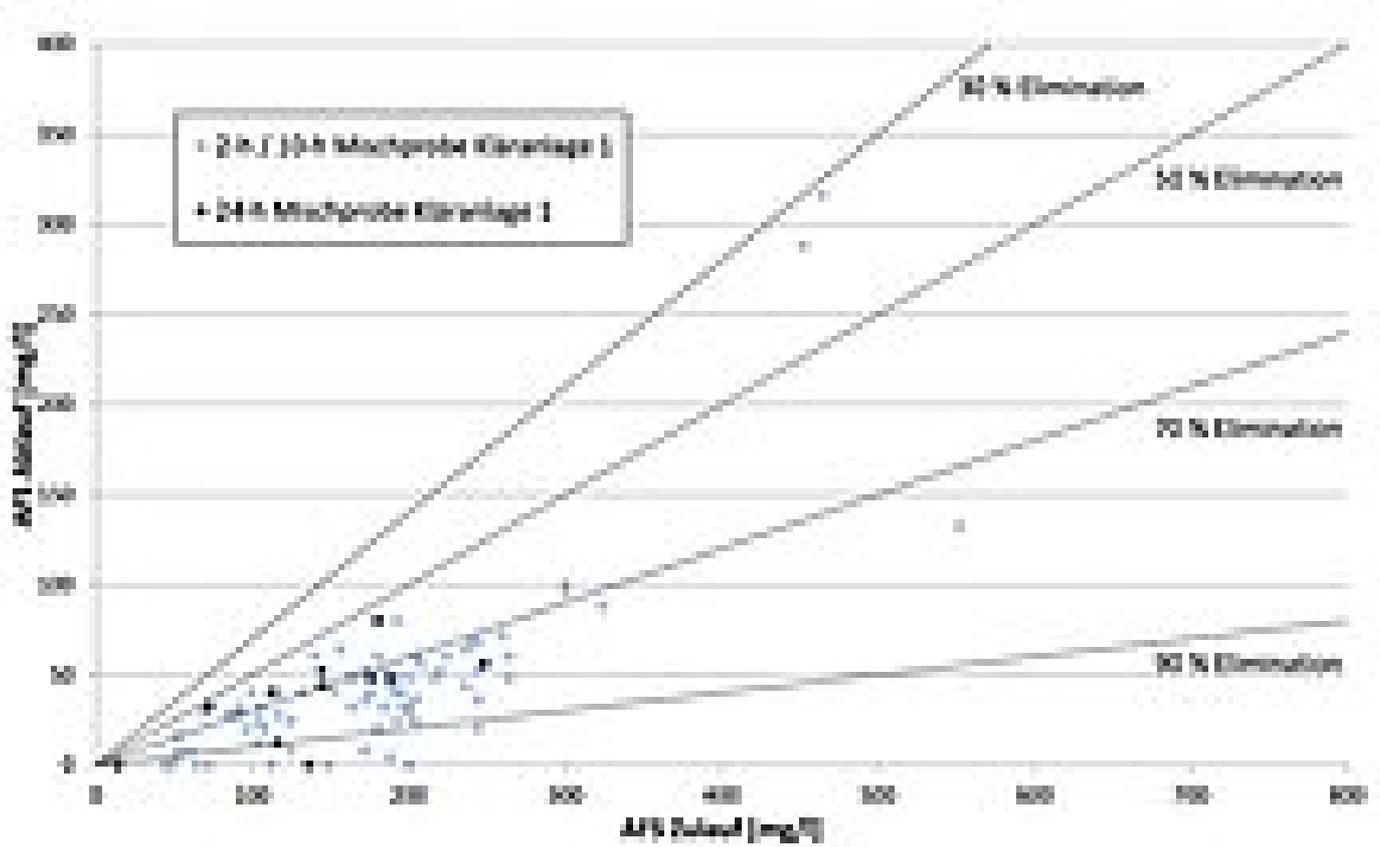
Reduction achieved for filterable solids with a plant size of 28,500 PE
