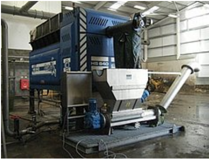
Wash Press / Compactor type WAP@ SL on trial
