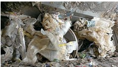
Rejects being turned over to drain free liquor
