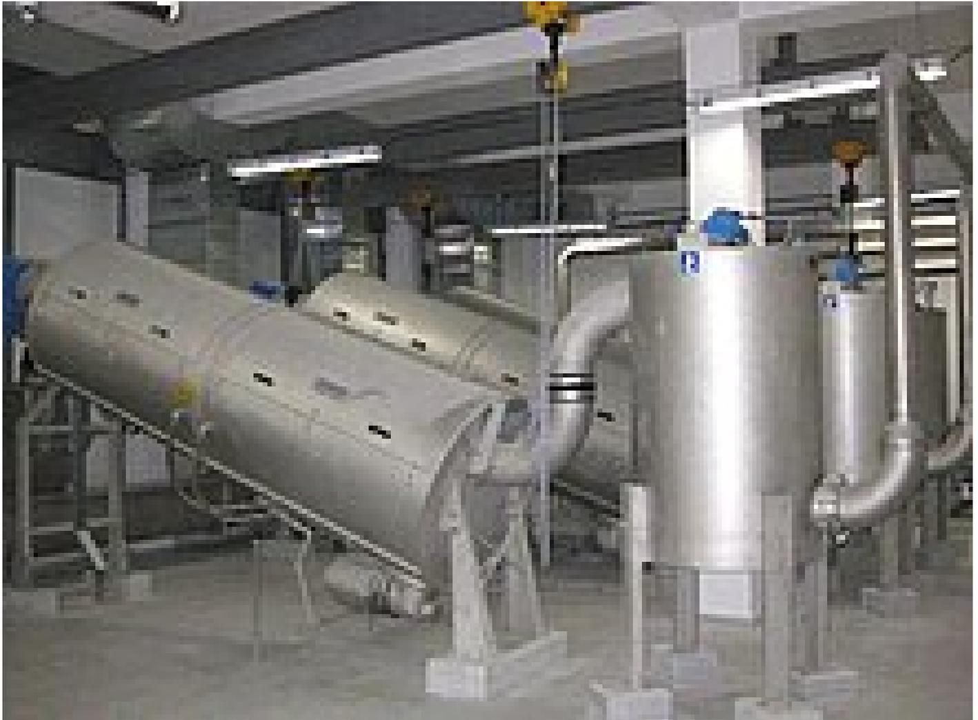
*Three ROTAMAT@ Screw Thickeners RoS 2 with upstream flocculation reactors*
