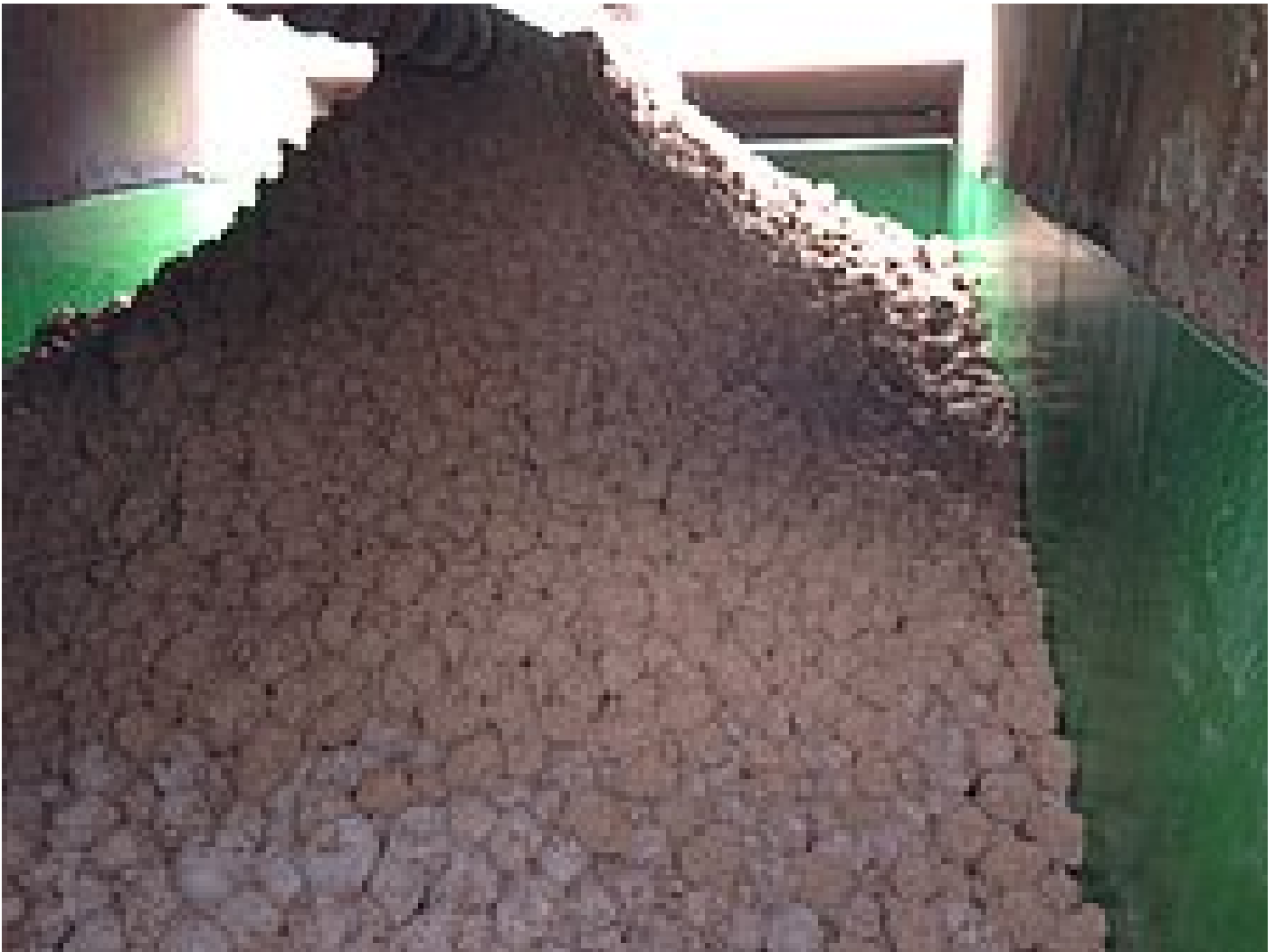
The cake from the Screw Press is consistently drier
