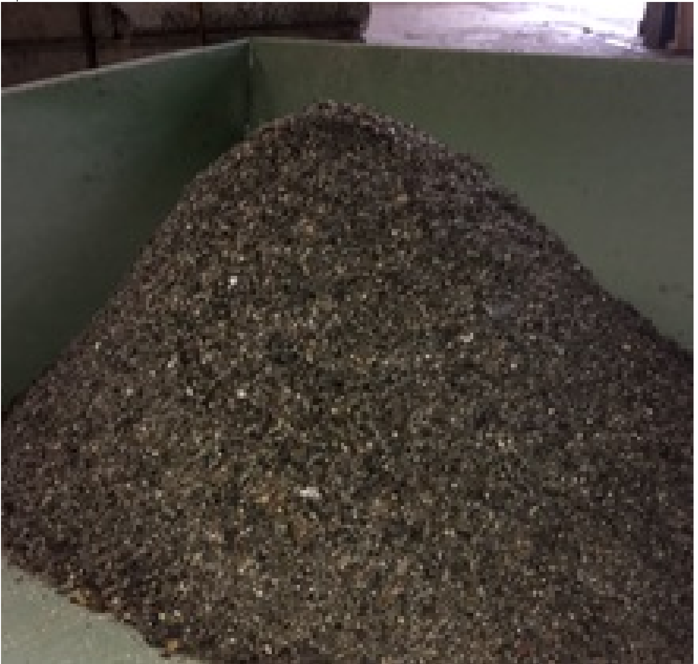
Figure 2: Removed and washed heavy medium / grit
