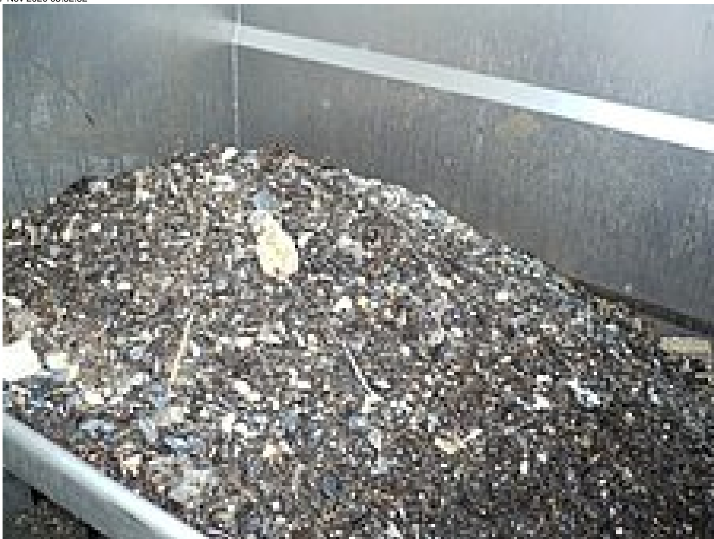
Removed coarse material subsequent to the Wash Drum
