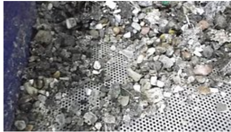
Sieved material removed from grit washer
