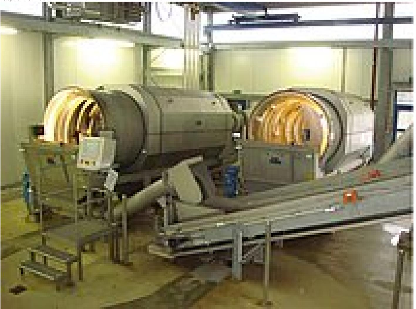
*Two ROSF 9 wash drums with WAP screenings presses for the removed and washed coarse solids*
