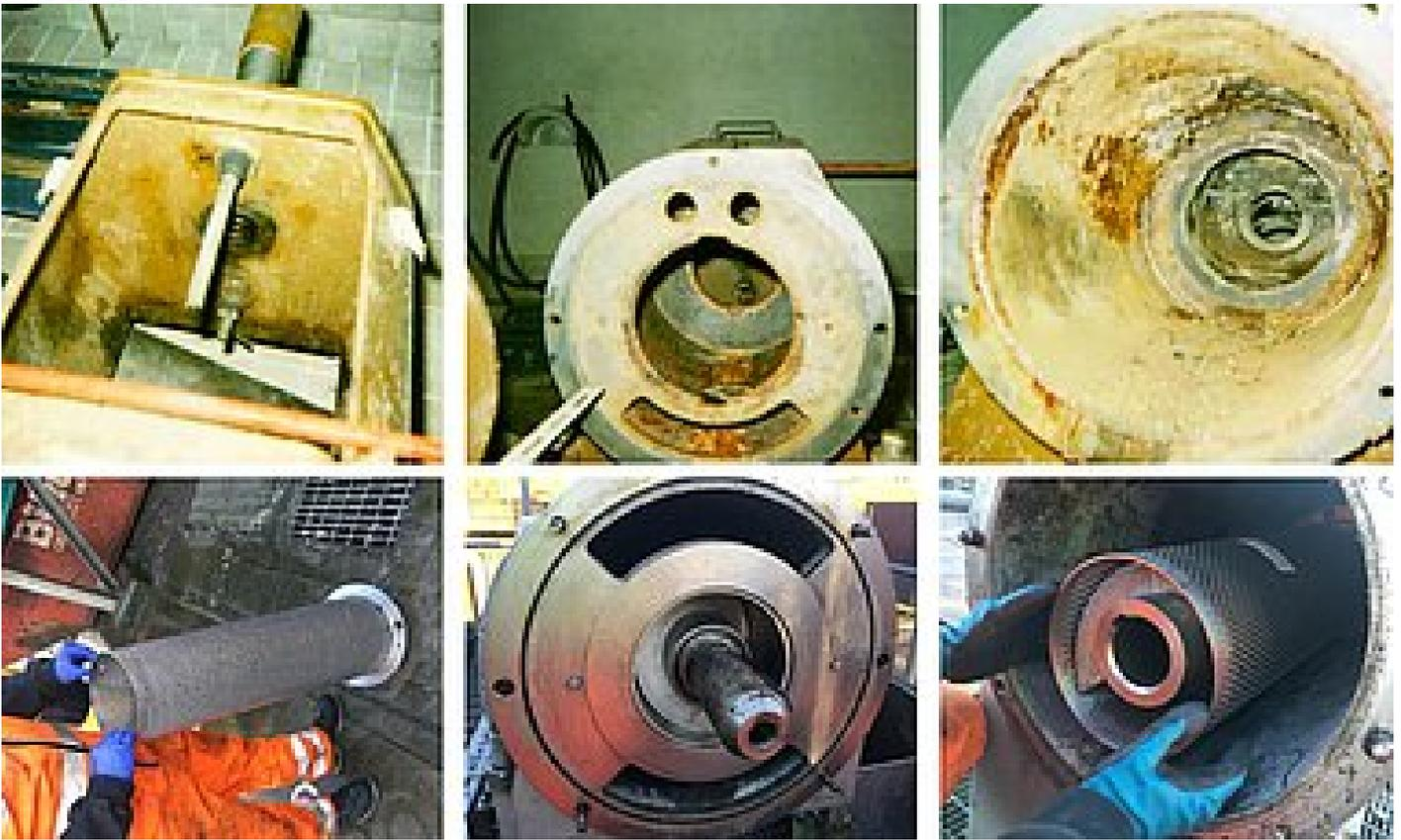
Figure 6. A comparison of various components of two similar sludge screens. The pictures above reveal components of a coated carbon steel screen with extensive corrosion after 12 years. The pictures below reveal components of a stainless steel screen after 12-13 years with no corrosion.
