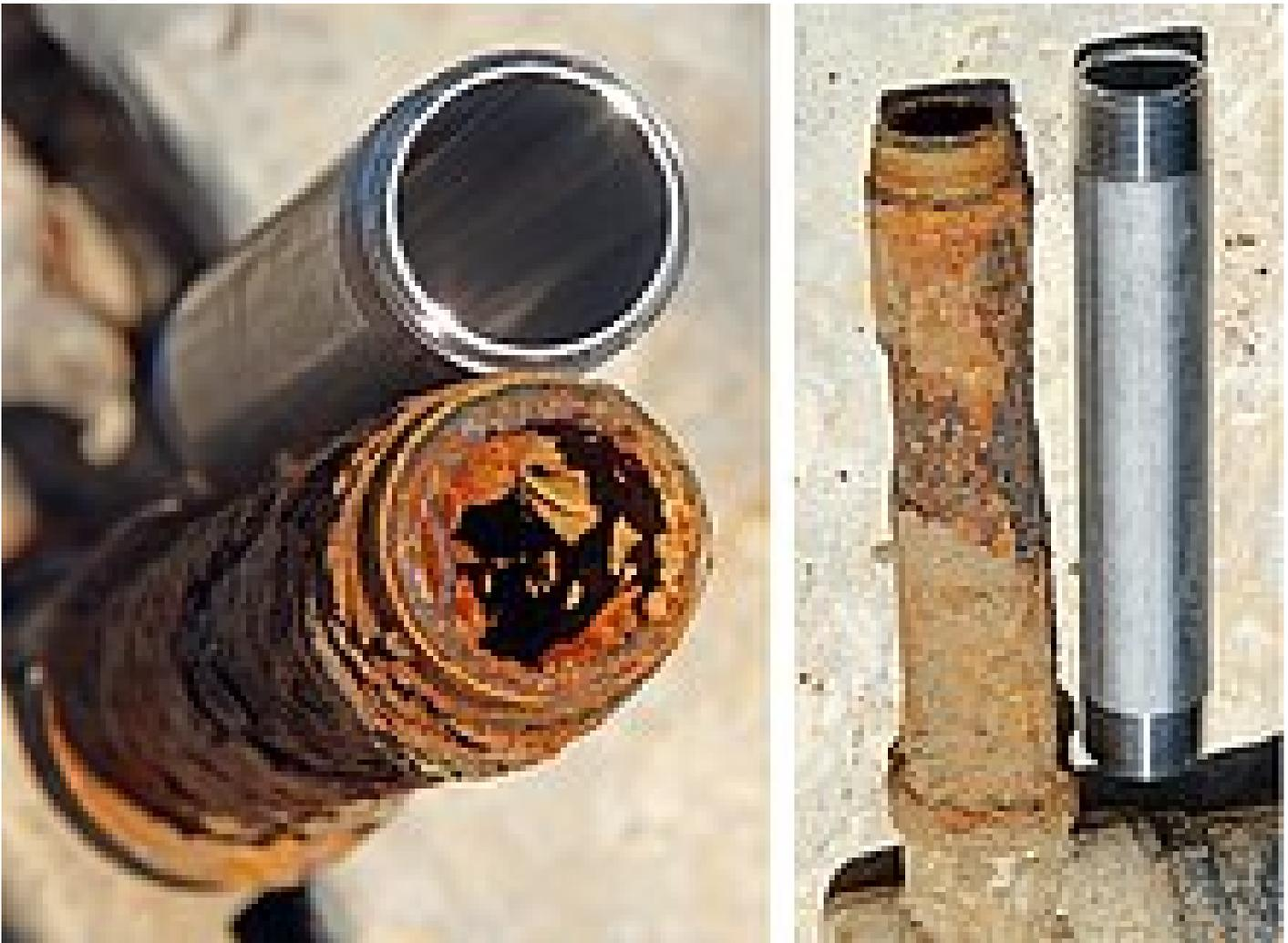
Figure 5. Extreme example of corrosion of a galvanised steel pipe after 6/7 years in a water supply system (TX, USA), compared to a stainless steel pipe (Raines, 2018)
