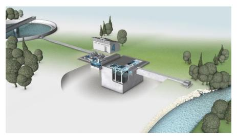
Fig. 16: HUBER has also developed solutions to treat water even further than usual. A so-called 4th treatment stage removes trace substances, such as pharmaceuticals, from the wastewater by adsorbing these substances to activated carbon.
