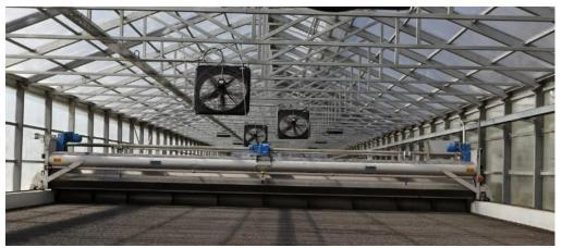
Fig. 30: Our HUBER Sludge Turner SOLSTICE<sup>®</sup> dries sludge in a glass house energy-efficiently with the power of the sun.
