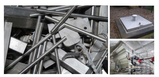
Fig. 19: HUBER manufactures products and machines for water and wastewater every year from approx. 4,500 t stainless steel. Reducing waste is a prerequisite for cost-optimised and resource-saving production when processing high-quality materials. HUBER therefore nests the parts to be manufactured from stainless steel with state-of-the-art CAM software for all orders. 100% of the stainless steel waste generated during production is recycled.
