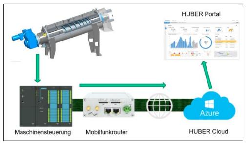
Fig. 10: Simplified principle of the HUBER Cloud Solution for operational support and process optimisation
