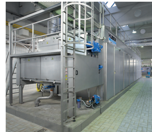
HUBER Belt Dryer BT 16 with condensation stage
