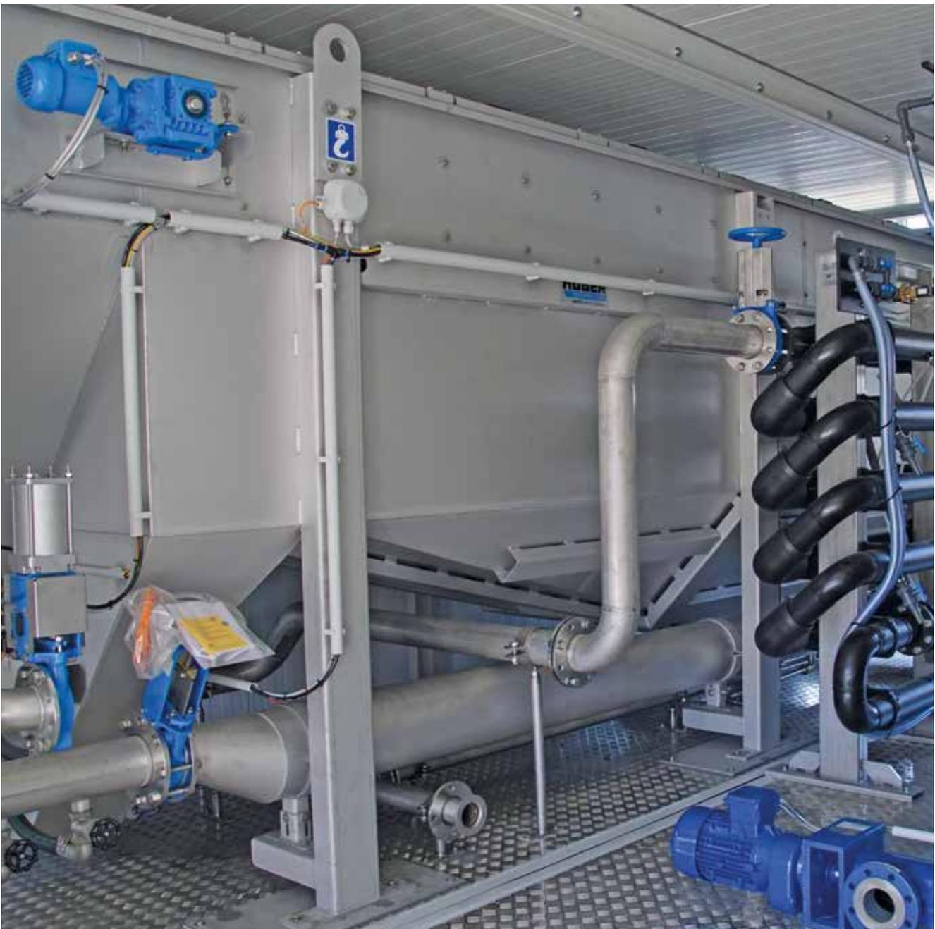
Installation in container construction up to 80 m<sup>3</sup>/h as a fast and mobile solution.
