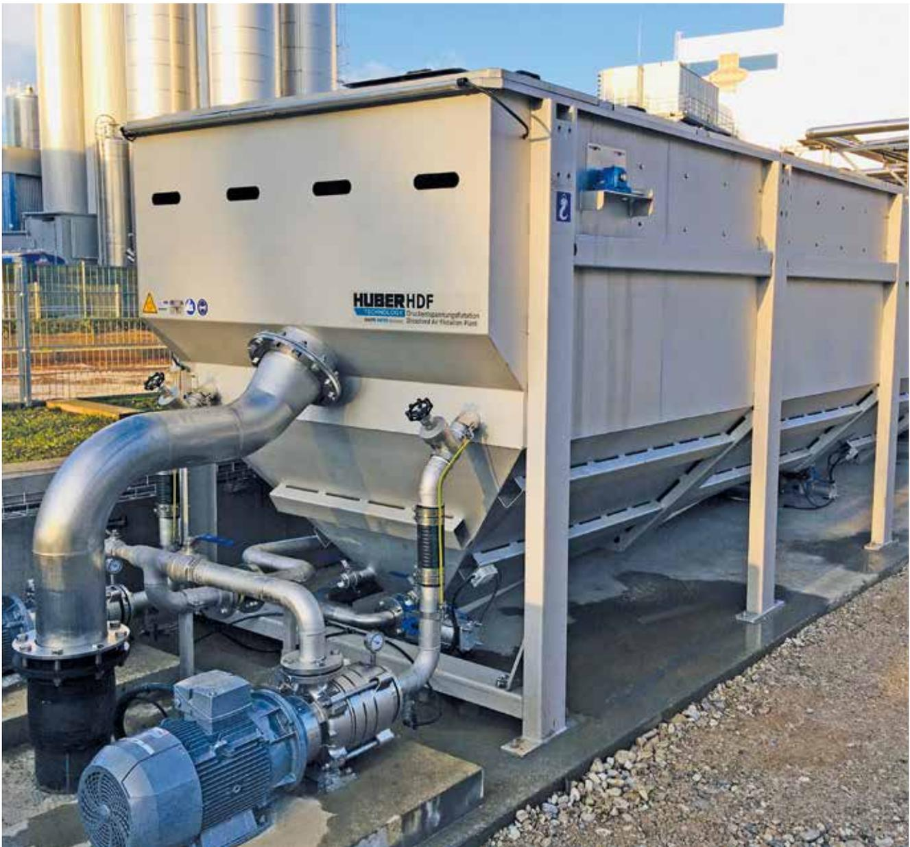
*HUBER Dissolved Air Flotation Plant HDF S installed for activated sludge separation.*
