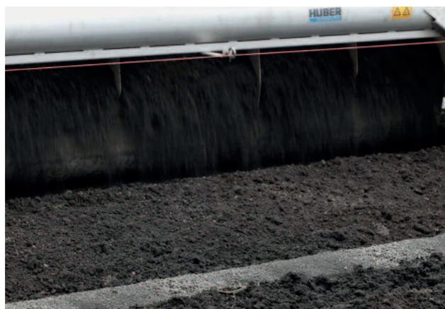
*With its shovel in horizontal position, the HUBER Sludge Turner SOLSTICE® can transport back dry sludge.*
