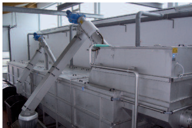
Odour-free, clean screenings and collected grit discharge
