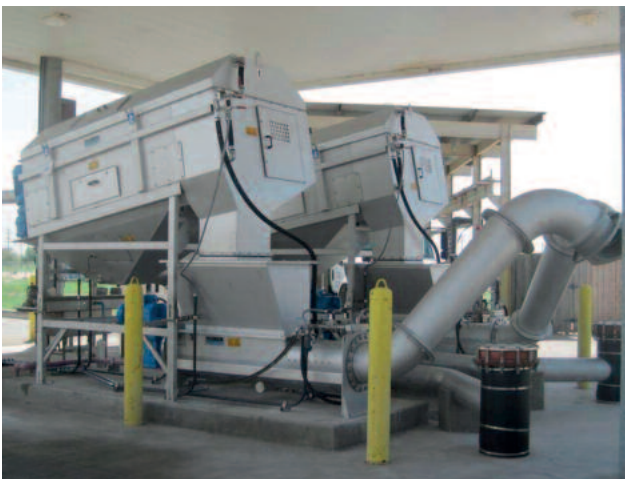
HUBER Wash Drum for washout and separation of all coarse material > 10 mm
