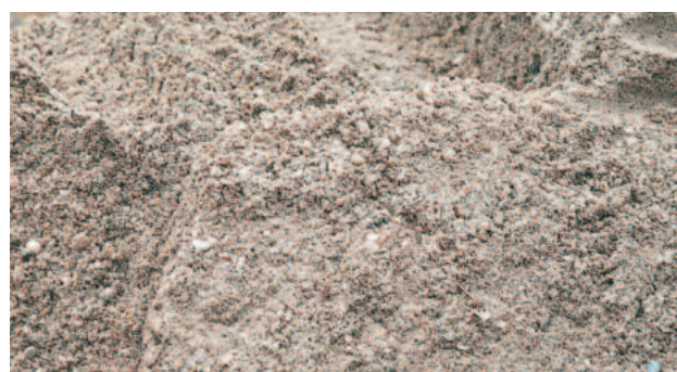
Washed grit removed at a wastewater treatment plant
