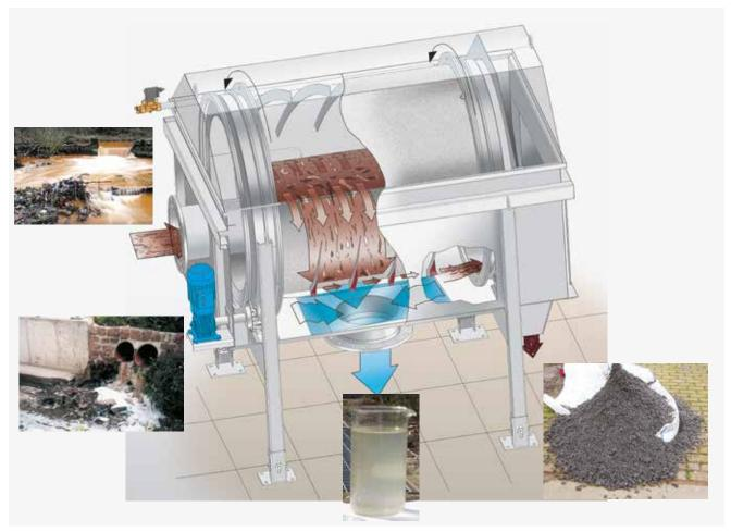
Schematic drawing of the HUBER Drum Screen RoMesh®.
