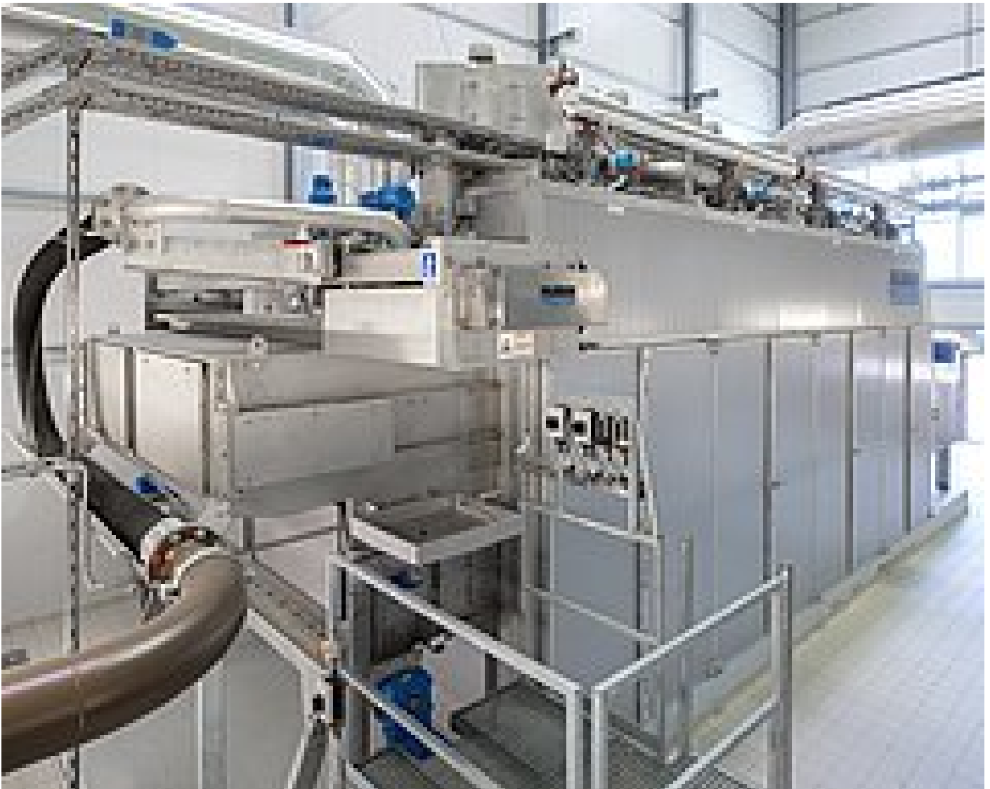
Fig. 2: HUBER Belt Dryer BT 8
