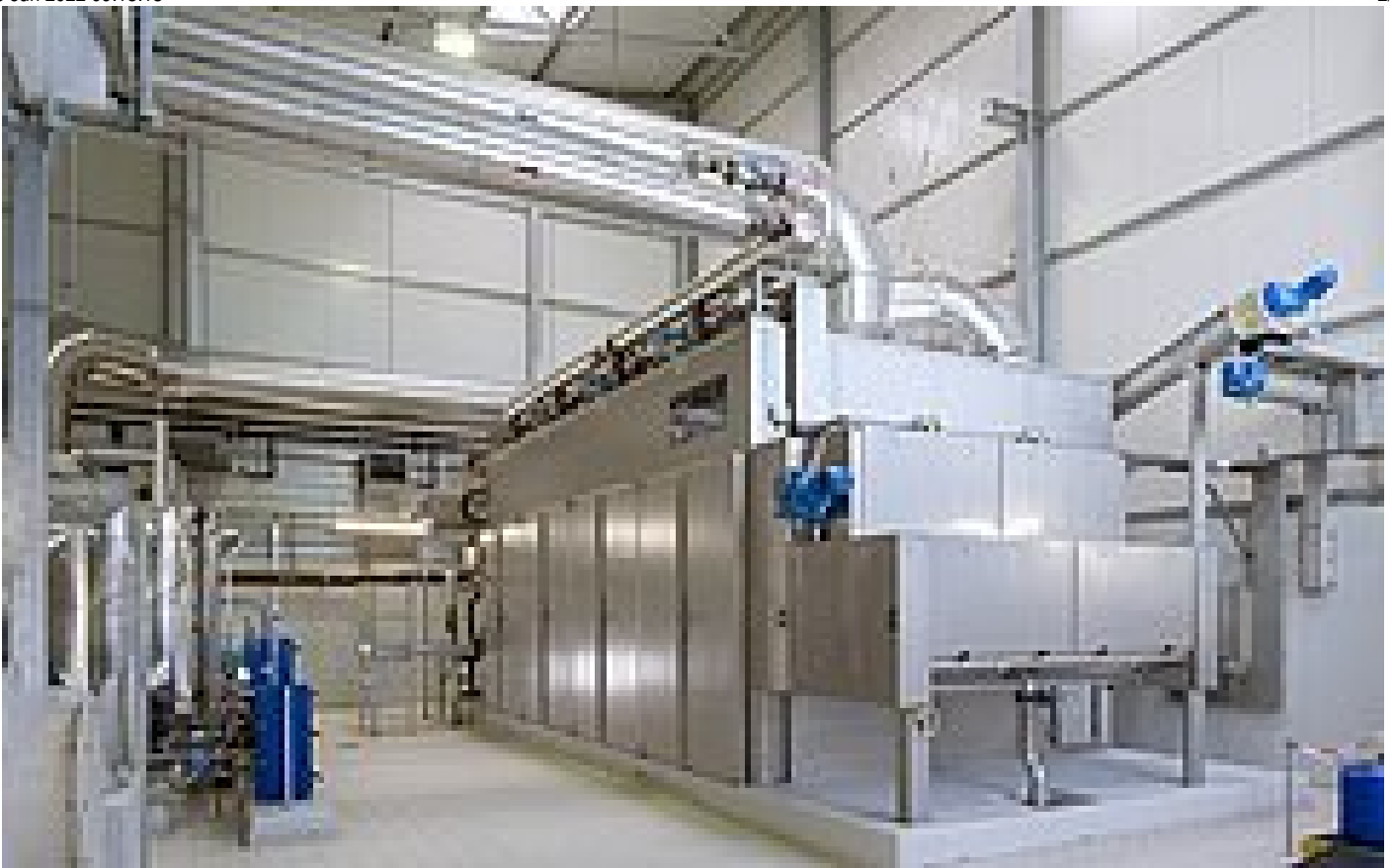
Fig. 2: HUBER Belt Dryer BT 8
