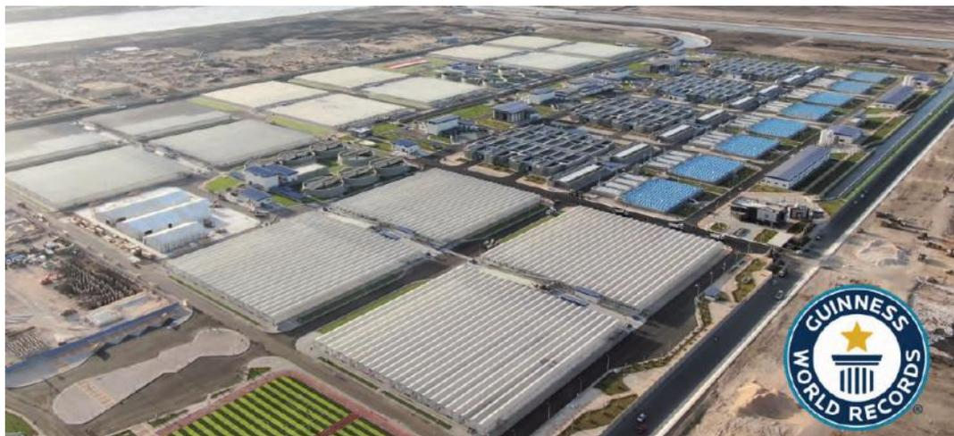
**Fig. 44: Clean water for the Sinai Peninsula: The water treatment plant in Bahr El-Baqar (Egypt) has recently been awarded by Guinness World Records as the world's largest plant of its kind. More than two billion cubic meters of water are to be treated here annually on an area of about 650,000 square meters. Among other things, HUBER supplied 128 SOSLTICE® sludge turners to dry 490,000 tonnes of dewatered sludge annually with the help of the sun.**
