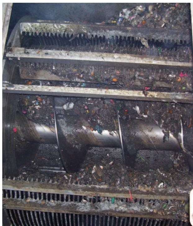
*In the fine screening plant undissolved solids are removed from the organic suspension (approximately 5 - 15 % of the inflow)*
