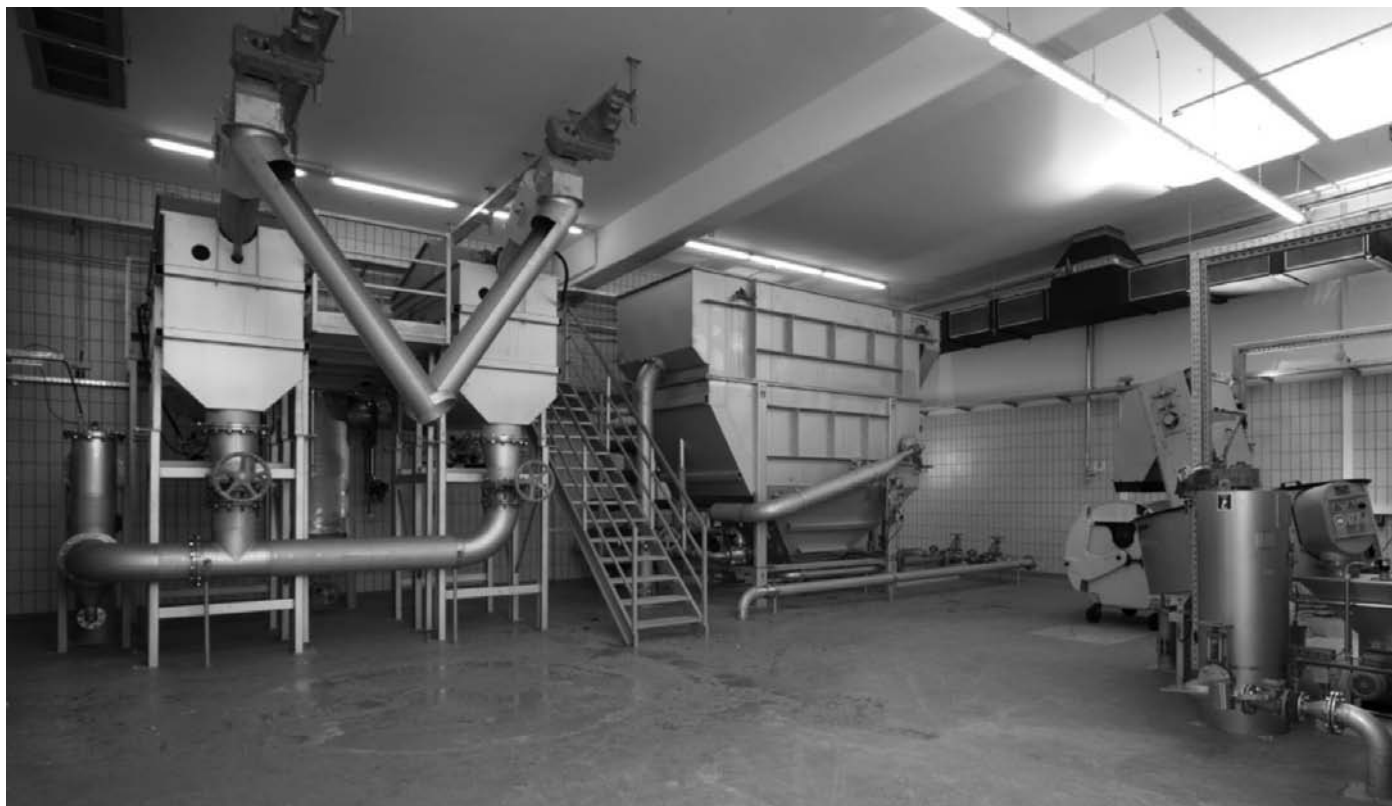
The pretreatment processes for the vacuum rotation membrane unit installed at a German meat processing facility include fine screens and a dissolved air flotation unit.
