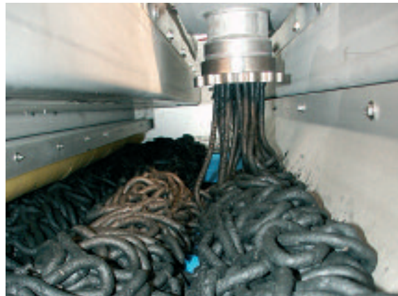
Sludge feeding through our extruder is essential for the outstanding performance of our belt dryers
