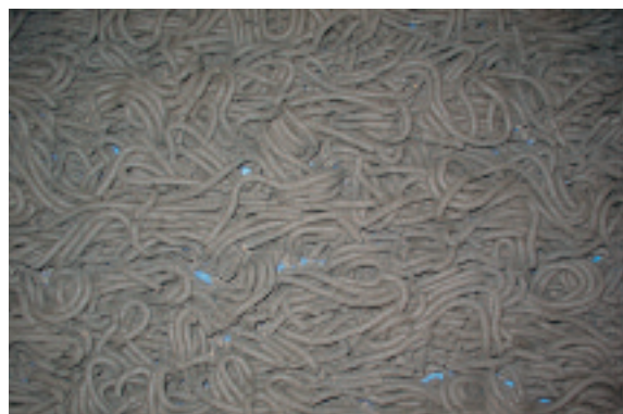
Porous sludge layer on the belt riding slowly and gently through the dryer; no mechanical stress is applied and virtually no dust generated
