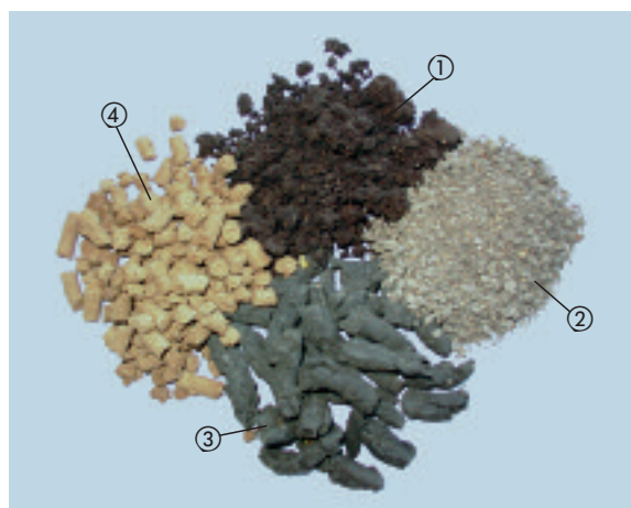
① aerobically digested sludge, fed through a pug mill; ② blended and comminuted industrial and municipal sludge; ③ anaerobically digested and extruded sludge; ④ extruded waterworks sludge
