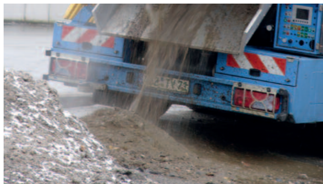
Untreated sewer grit
