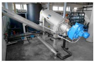
HUBER Screw Press Q-PRESS<sup>®</sup> for process sludge dewatering in tanneries.
