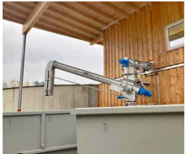
Containers are filled by the Ro8 TC with automatic chute and automatic swivel drive.
