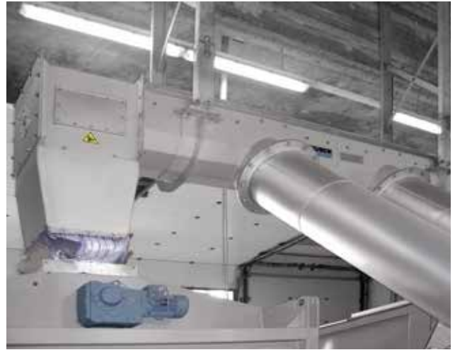
Ceiling-mounted distributor for pressed screenings with two end discharge units.
