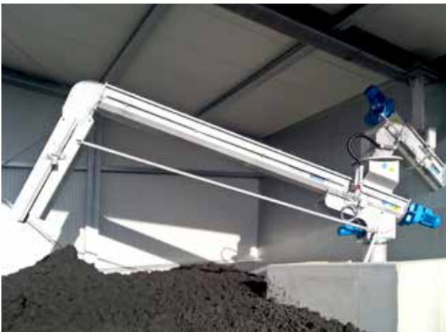
Rotating Distribution Screw Ro8 TC for dewatered sludge to supply open areas or containers.
