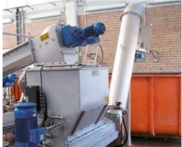
HUBER Screw Conveyor Ro8 T discharging screenings into a HUBER Wash Press WAP® SL.
