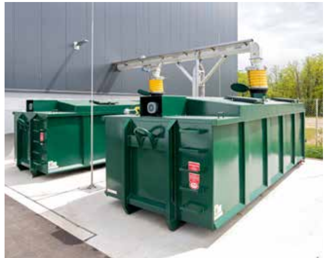
HUBER Trough Screw Conveyor Ro8 T for a fully enclosed disposal solution with loading bellows.
