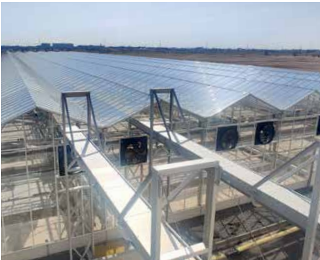
HUBER Trough Screw Conveyor Ro8 T as supplying conveyor bridge to a HUBER Solar Sludge Dryer .
