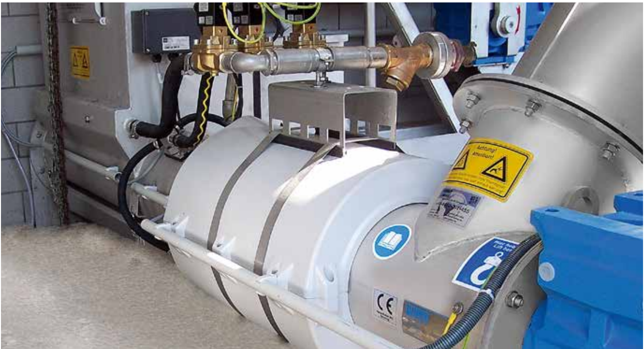
HUBER Screenings Compactor Ro7 – compact design, with optional screenings washing.
