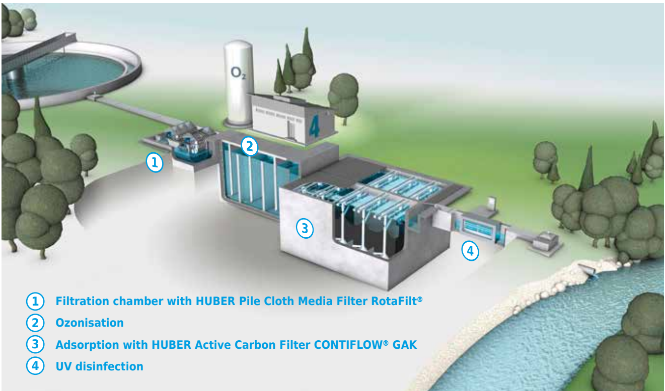
Variant 1: Combination of ozonisation with subsequent activated carbon filtration (GAK), upstream cloth filtration (police filter) and downstream UV disinfection.
