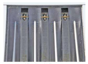
Backwashing of filter discs with filtrate – no external wash water required.
